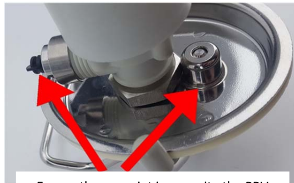
Ensure the spray jet is opposite the PRV
